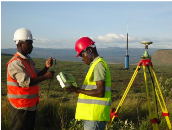
Photo 4: Use of GPS for Detail Picking
